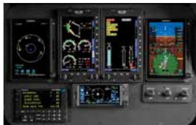
Glass Cockpit with Howell Instruments Engine Instruments Display & Garmin G500TXi MFD/PFD
