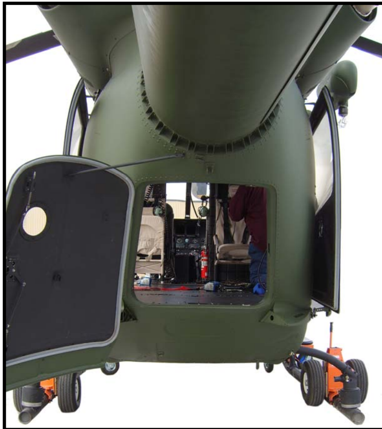
The MD 902 Explorer Baggage Compartment Area Can be Configured for Alternative Loading Capabilities
